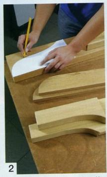
Create a curved profile template. Use the same template to mark the curve profiles on the base rail, back rail and front leg. Cut along the profile lines with a jigsaw or band saw.
