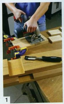
Mark the area on each piece that will overlap. Set the saw blade depth to half the thickness of the stock. Make several passes, starting at the inside edge of the half-lap area.
