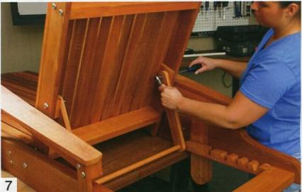
Attach the back assembly to the base assembly with bolts, washers and locknuts. Then attach the support arms to the back frame.
