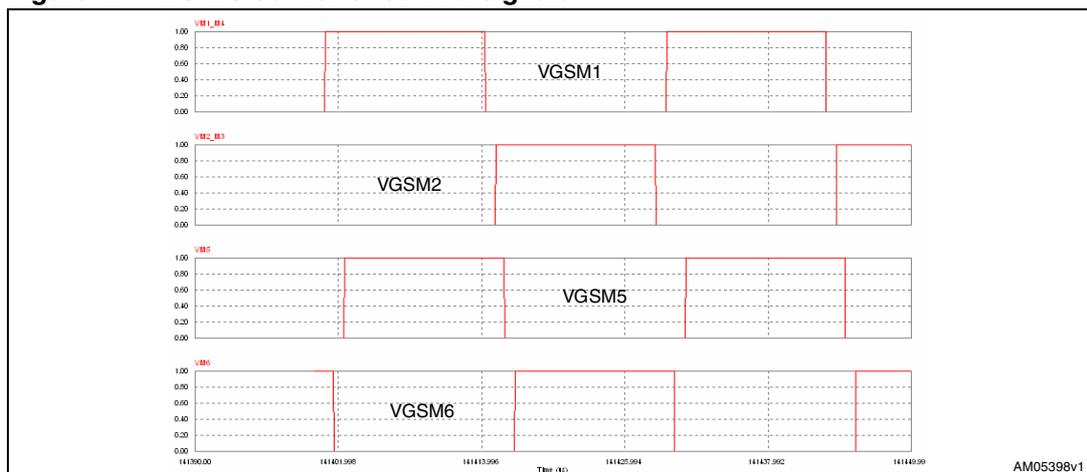
The same drive signal used for device M1 also controls M4, as the one controlling M3 is also used for M2. The effect of the input bridge modulation is to generate a square wave on the
