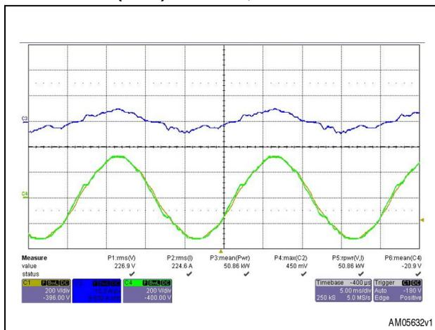
**Figure 39. Inverter voltage (green) and current (yellow) at 2500 W, PF**
