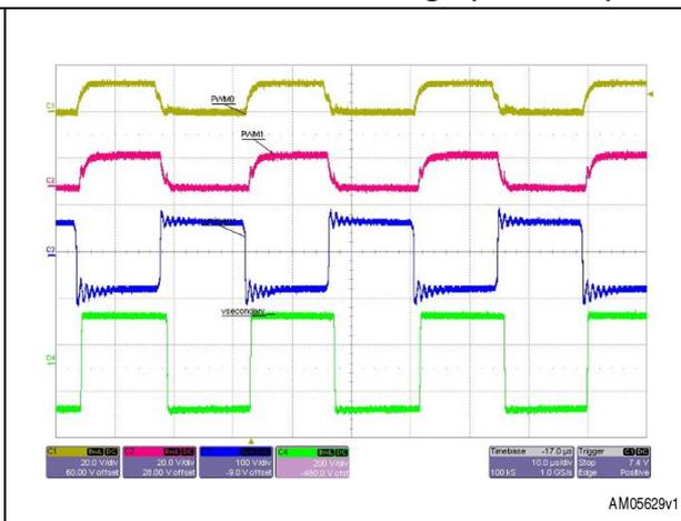
The PWM embedded peripheral used for the DC-AC stage is configured to generate a triangular carrier at 17.4 kHz with a resolution of 16,6 ns and programmable dead-time insertion to avoid cross-conduction. For the sake of security the complementary pairs must be disabled synchronously in the case of power stage failure/fault (e.g. overcurrent) and this is performed by a dedicated emergency stop input embedded in the peripheral.
