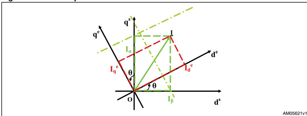
The difference between reference components of the current and the actual DQ components are the inputs of the PI regulators in the inner control loop. The outputs of the PI regulators in the inner loop are two voltage components,  $V_d$  and  $V_q$ . By performing a reverse park transformation, two AC voltages are generated back to the stationary reference frame, and therefore the generation of the modulating signals of the DC-AC converter may be executed by the microcontroller.
