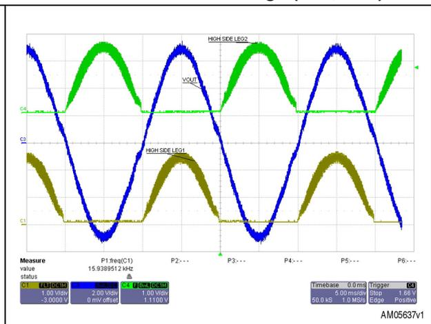
Figure 44. Low-side device modulation (red and blue track); high-side device modulation (yellow track and green track)
