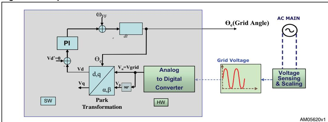
The grid voltage and the 90° phase-shifted voltage are used to perform the reference frame change, or “park transformation”, and create two voltage components on the DQ reference frame called  $V_d$  and  $V_q$ . One of the two components is controlled to zero with a PI regulator. The output of the PI regulator is the grid frequency which may be integrated to obtain the grid angle.
