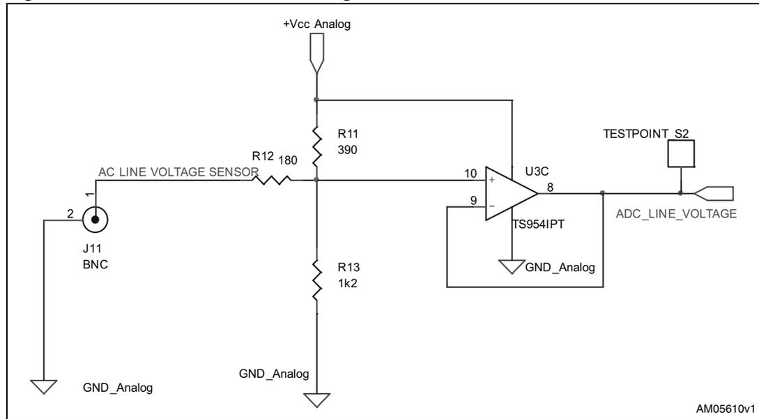
The circuit is supplied by the 5 V bus generated by the multi-output power supply and the measured voltage is fed through connector J11. The output voltage of this circuit is then equal to the sum of the measured voltage plus an offset voltage according to the following equation:
