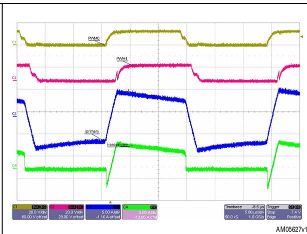
Figure 34. Power MOSFET M1- Ch1 gate signal; Ch2 drain-source voltage and drain current Ch4
