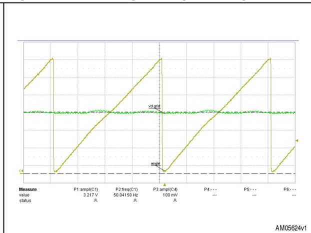
Figure 31. Grid angle (yellow), grid voltage (red), 90° phase-shifted voltage (blue)
