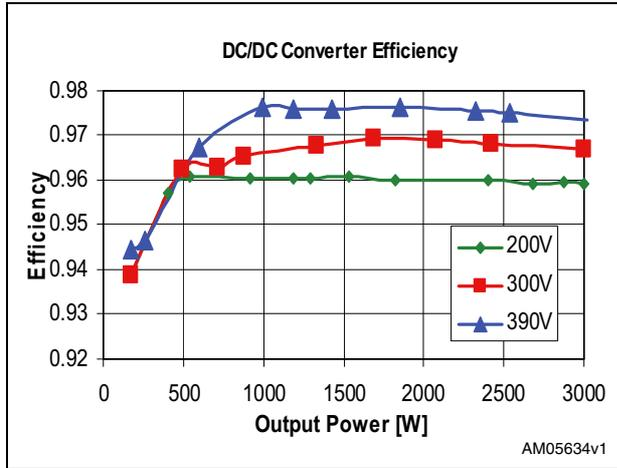
Figure 41. System efficiency
