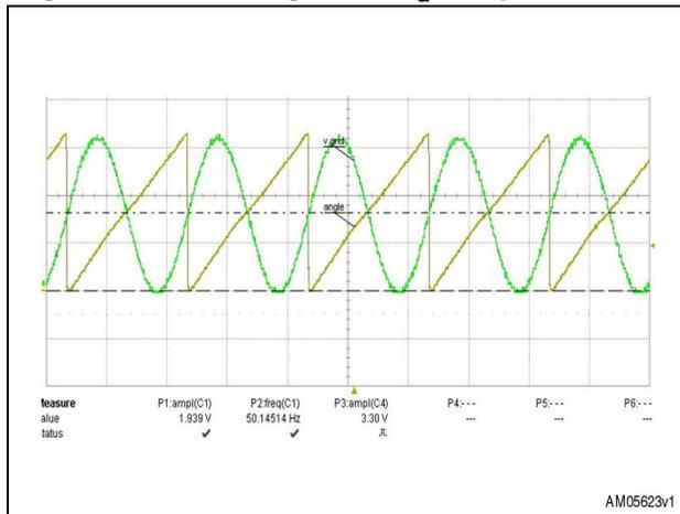
Figure 30. Grid angle and grid voltage
