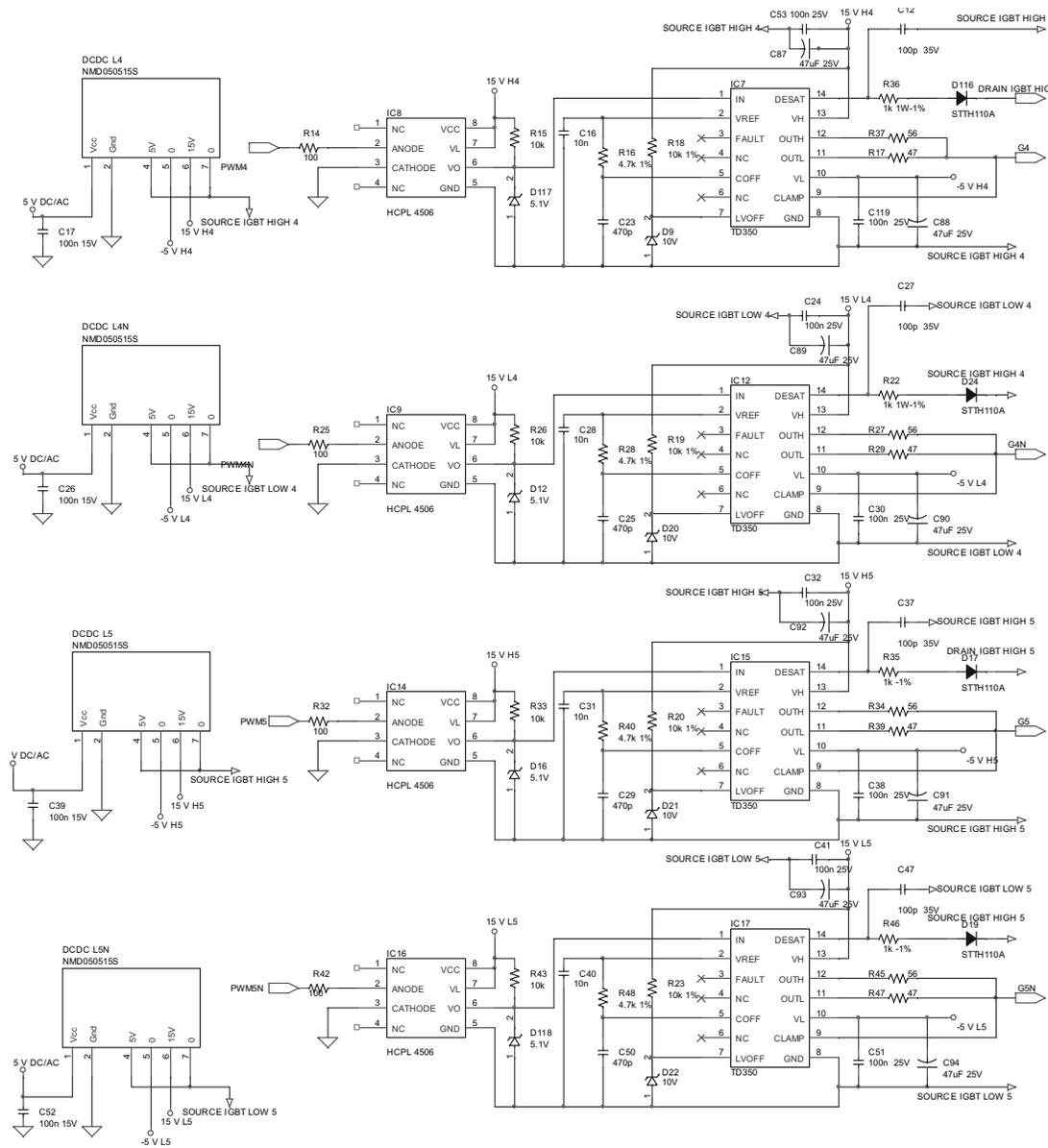
The outputs of the microcontroller are the PWM signals used to control the power devices in each leg of the conversion system.
