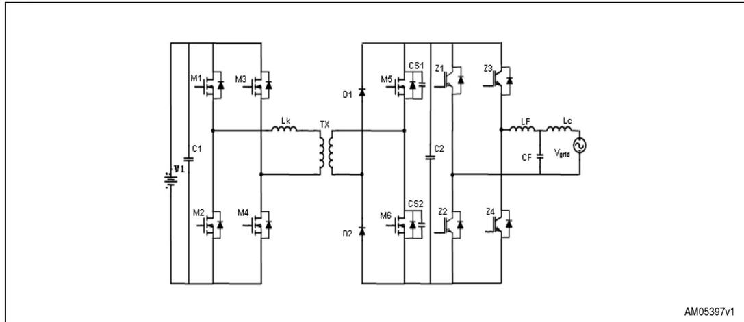
The DC-DC converter is depicted in *Figure 3* together with the DC-AC converter and LCL filter. The converter consists of an input capacitor, C1, six switches, M1 - M6, six freewheeling diodes, two rectifier diodes, D1 and D2, a HF transformer with turns ratio equal to 1.2 and a DC link capacitor C2.
