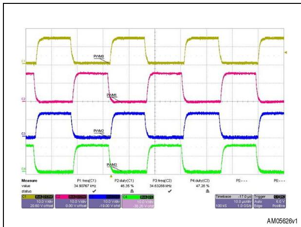
Figure 33. Phase-shifted signals, transformer current in CCM, power MOSFET M1 drain current
