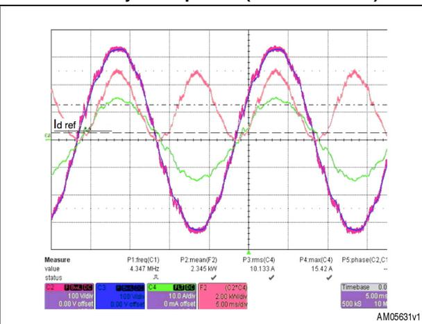
**Figure 38. Inverter voltage (green) and current (blue) at 800 W, PF=0.97**
