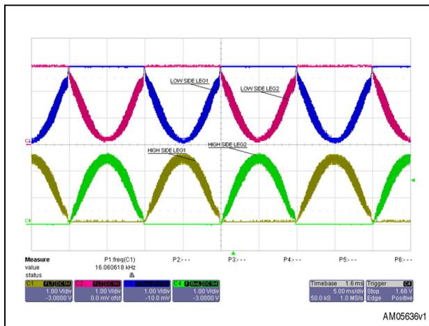
Figure 43. Phase-shifted gate signals (Ch1, Ch2), primary and secondary transformer voltage (Ch3, Ch4)
