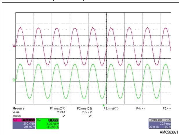
**Figure 37. Grid voltage (blue), inverter voltage (red), injected current (green); injected power (math function)**
