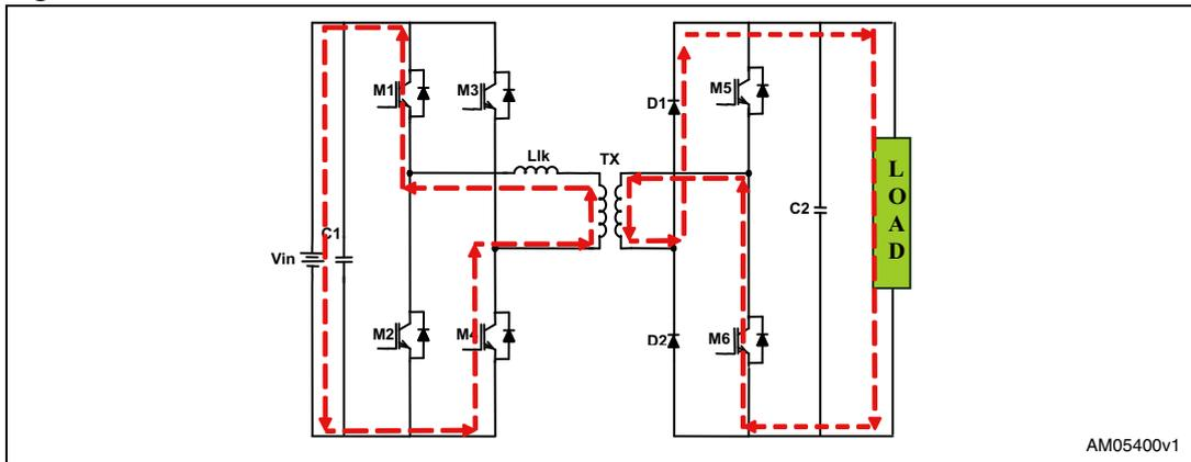
This mode ends when leakage inductor current reaches zero at  $t=t_1$ .
