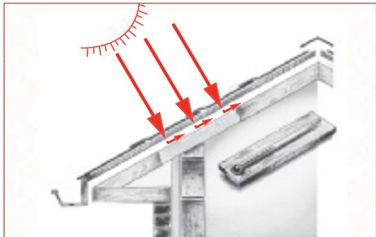
**Ventilated:** lower temperature inside. With air gap between insulation and roof deck: air escapes via ridge vents, leaving the roof structure unaffected.
