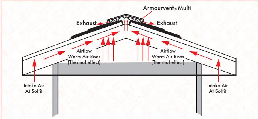
The most important factor in roof ventilation is the need for a “balanced system”. This means for every cm<sup>2</sup> of air exhausted, it must be balanced by providing the same amount of air intake at the eaves.
