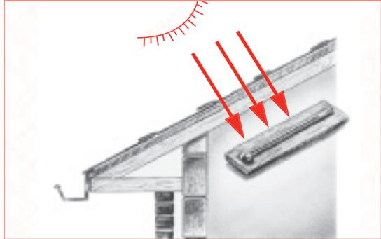
**Unventilated:** high temperature inside. Without air gap between insulation and roof deck: condensation forms and the roof structure is damaged.
