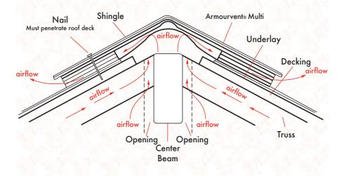
Detail: Armourvent® Multi on ridge application. (double beam)
