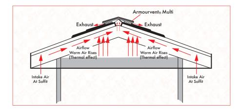
The most important factor in roof ventilation is the need for a "balanced system". This means for every cm<sup>2</sup> of air exhausted, it must be balanced by providing the same amount of air intake at the eaves.
