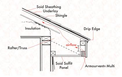
7 Detail: Armourvent® Multi eave application. (narrow overhang)
