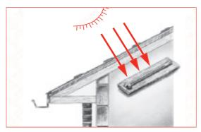
**Unventilated:** high temperature inside. Without air gap between insulation and roof deck: condensation forms and the roof structure is damaged.
