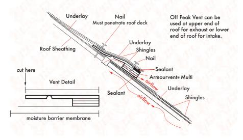
5 Detail: Armourvent® Multi shed roof application
