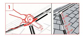
inlength, spaced with a 30 cm uncut area between each 45 cm opening. The slot for ventilation should not be cut any lower than 1/3 of the roof to maintain a balanced ventilation system.
