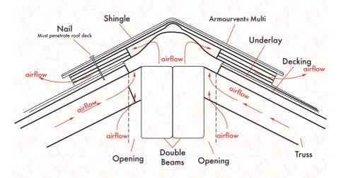
Detail: Armourvent® Multi off peak application (intake or outlet)
