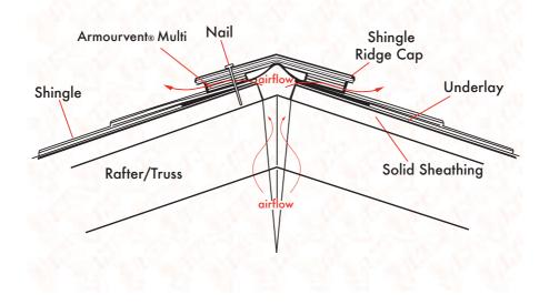
2 Detail: Armourvent® Multi on ridge application. (single beam)
