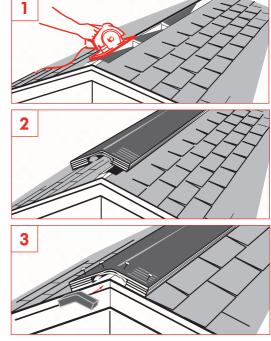
cap. Multiple lengths of vent can be joined by butting the sections tightly together. We require applying IKO Shingle Stick® to the shingles, before installing the vent on the ridge. This sealant should fill any voids between the bottom of the vent and the surface of the shingle.
