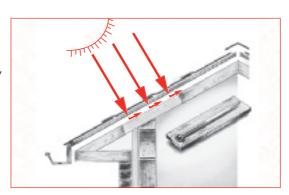
Ventilated: lower temperature inside. With air gap between insulation and roof deck: air escapes via ridge vents, leaving the roof structure unaffected.
