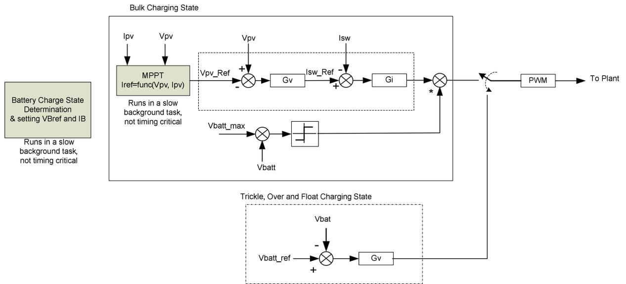
**Fig 7 Battery Charging with MPPT Control Diagram**
