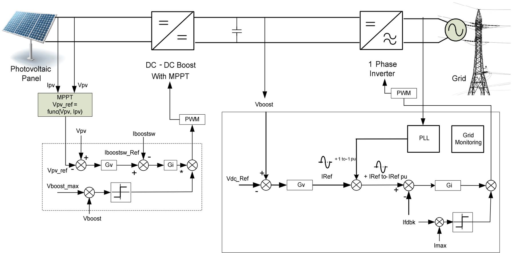
**Fig 12 Control of PV Grid Tied Inverter**
