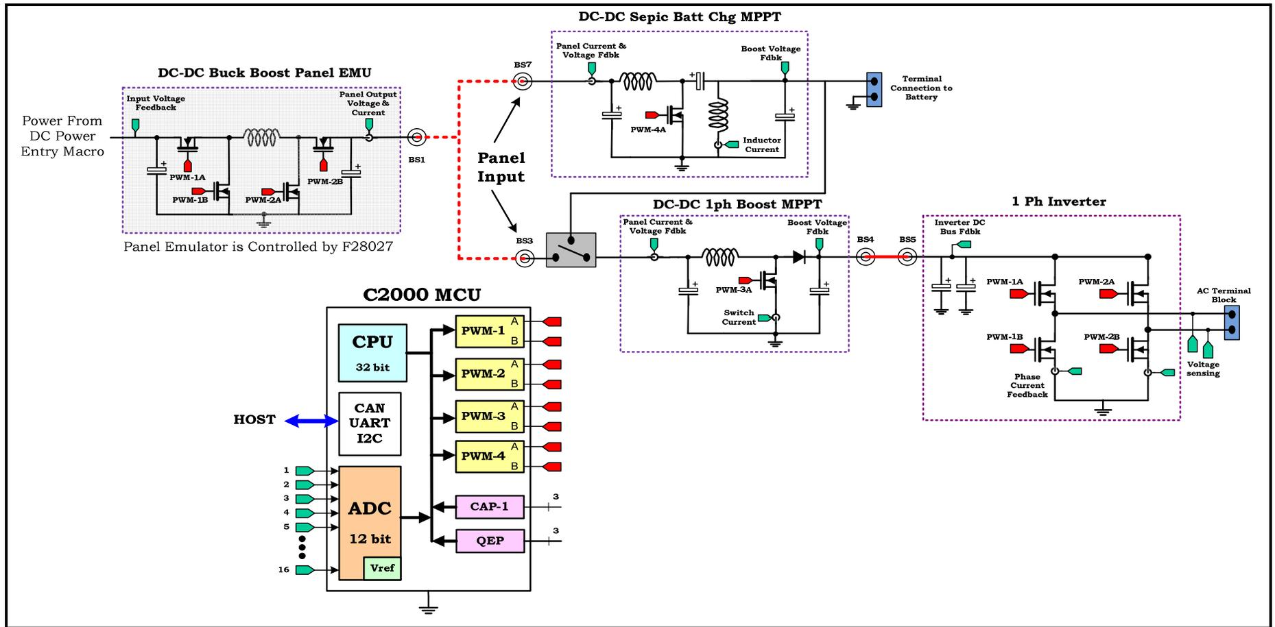
Fig 15 Solar Explorer Kit Block Diagram with C2000 MCU
