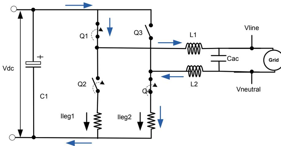
Primary Current fed into the grid during the positive half is  $i_{leg2}$ ,  $i_{leg1}$  will measure zero. However when the current reference for the inverter is very low i.e. Q1 is open most of the times, this can result in shorting the grid across SW2 and SW4. When shorted a high current flows through both Leg1 and Leg2. This is why the Leg1 current is subtracted from the Leg1 current at all times to get the change in the grid current.
