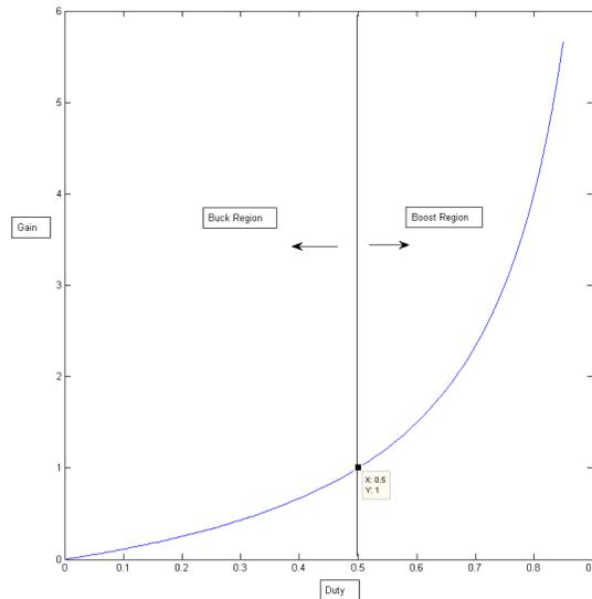
Therefore it can be concluded for duty less than 50% the stage behaves as a buck and 50% and above as a boost. The detailed switching diagram using C2000 PWM module is depicted below.
