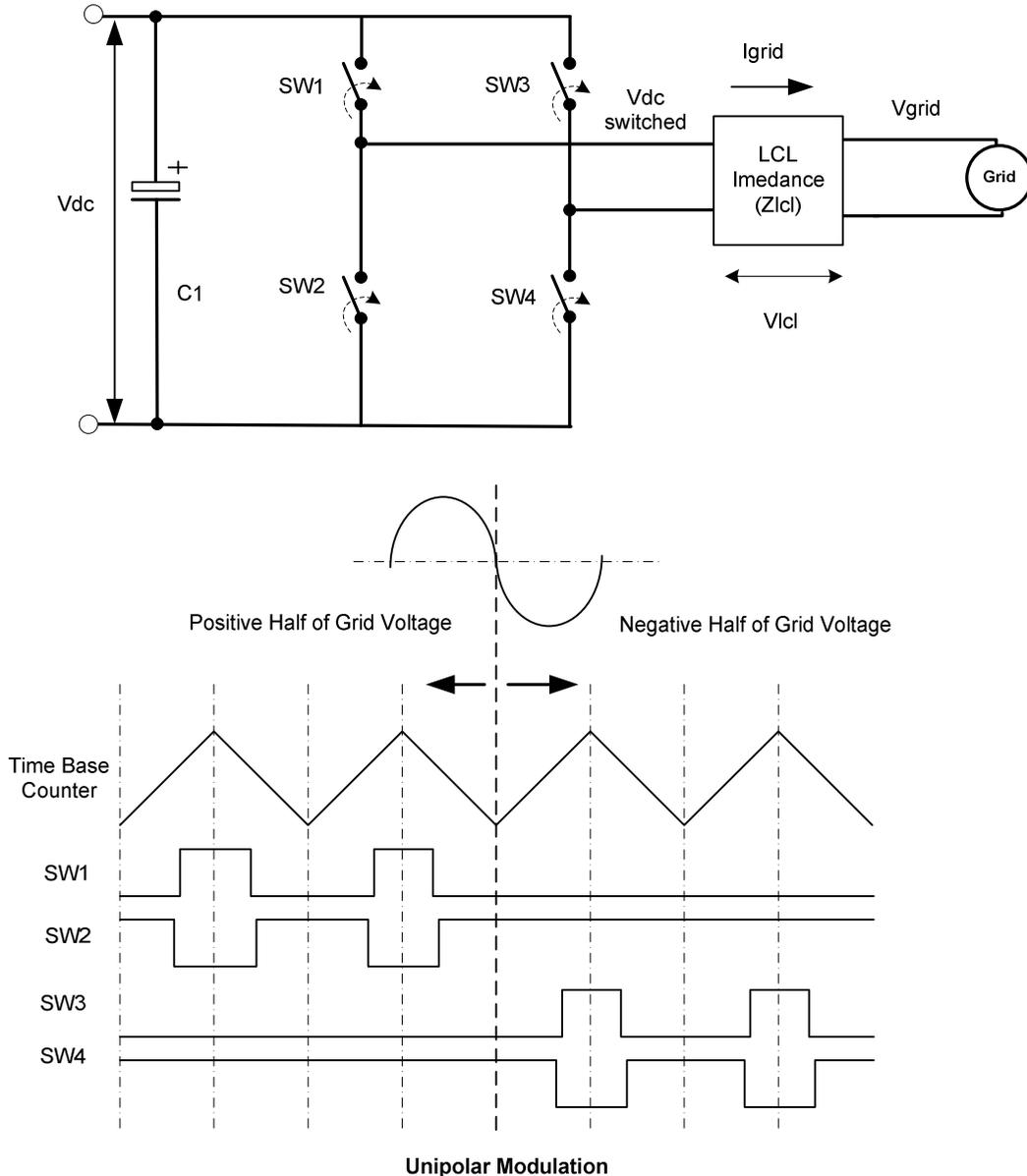
LCL filter at the output of the inverter filters this waveform. Now the voltage across the LCL filter can be written as
