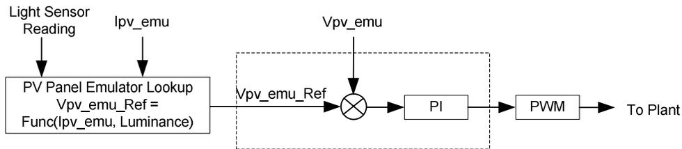
The current being drawn by the panel  $I_{pv}$  is used as the index for the look up table that is stored on the controller. The look up table is then used to provide the voltage reference  $V_{pv\_ref}$  for the panel corresponding to the  $I_{pv}$ . A light sensor is placed on the board to control the irradiance level and produce a corresponding V-I curve. For getting curves
