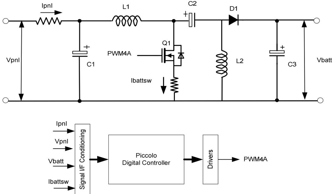
**Fig 6 DC-DC Battery Charging Sepic Power Stage**
