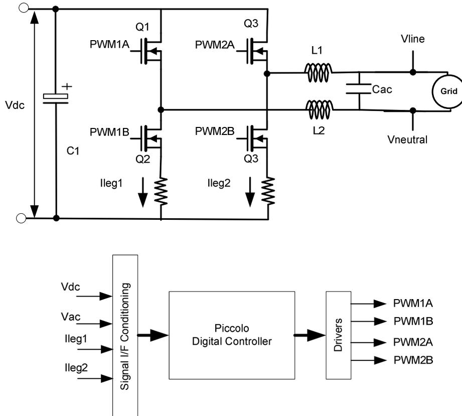
Fig 8 Single Phase Full Bridge Inverter Power Stage
