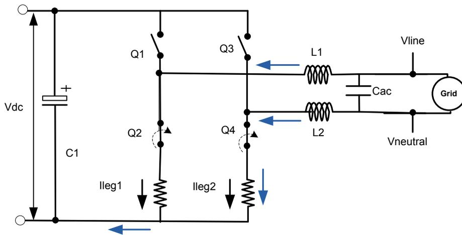
Shorting the grid under low modulation case, then negative current is not sensed.
