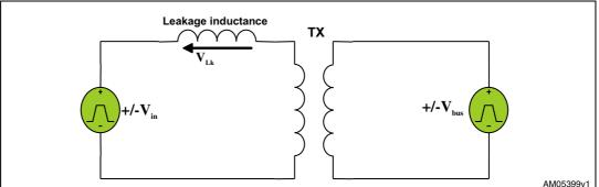
As a result, the primary voltage and the secondary transformer voltage reflected to the primary determine the rising and falling slope of the current in the leakage inductance. According to leakage inductance current waveforms, two operating modes may be distinguished for the converter:
