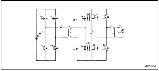
The DC-DC converter is depicted in *Figure 3* together with the DC-AC converter and LCL filter. The converter consists of an input capacitor, C1, six switches, M1 - M6, six freewheeling diodes, two rectifier diodes, D1 and D2, a HF transformer with turns ratio equal to 1.2 and a DC link capacitor C2.
