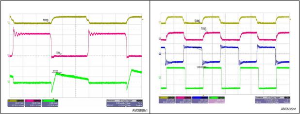
The PWM embedded peripheral used for the DC-AC stage is configured to generate a triangular carrier at 17.4 kHz with a resolution of 16,6 ns and programmable dead-time insertion to avoid cross-conduction. For the sake of security the complementary pairs must be disabled synchronously in the case of power stage failure/fault (e.g. overcurrent) and this is performed by a dedicated emergency stop input embedded in the peripheral.
