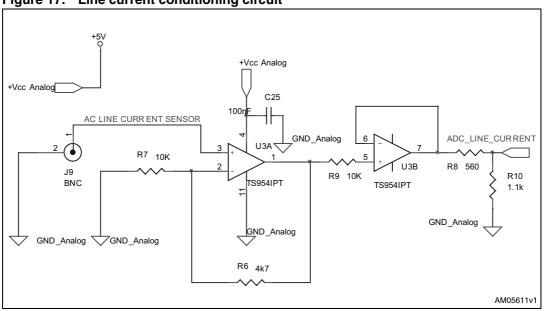
Figure 17. Line current conditioning circuit
