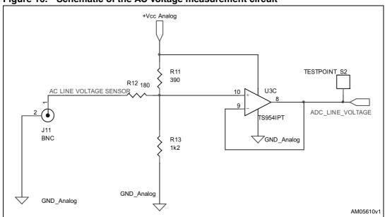
Figure 16. Schematic of the AC voltage measurement circuit
