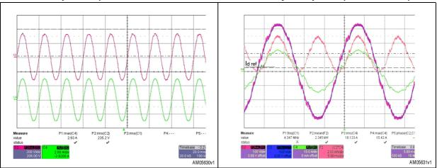
Figure 38. Inverter voltage (green) and current Figure 39. Inverter voltage (green) and current (blue) at 800 W,PF=0.97
