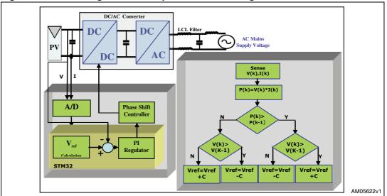
Figure 28. Block diagram of the implemented MPPT algorithm
