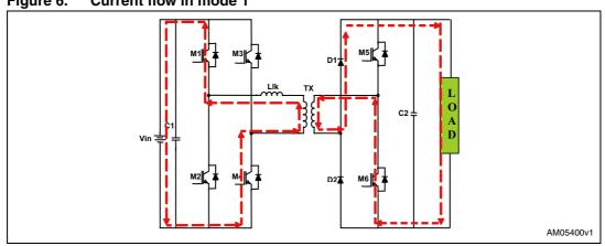
Figure 6. Current flow in mode 1
