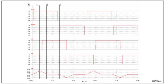
Figure 10. Modulation and transformer current in DCM
