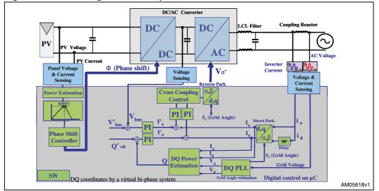
Figure 24. Block diagram of the implemented control
